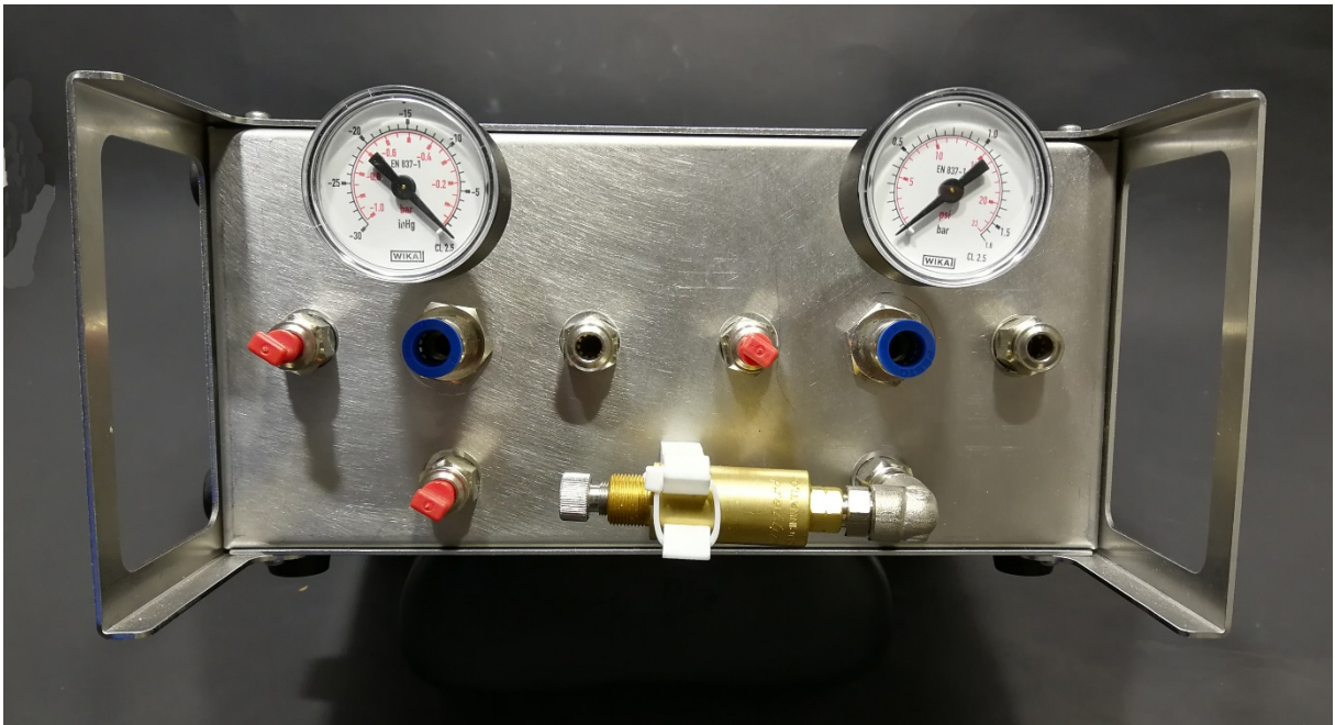
Photo show vacuum connected to the left channel and pressurised air to the right channel.
