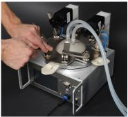
Erato mounted with Thorax dome/Pericardium membrane in Hephaestus cabinet. 8 stainless steel quick release couplings gives easy access for exchange. The hoses connected to Thorax dome perform as hose valves controlled by two ACRO 933 pneumatic pinch valves (Mitral and Aortic).
